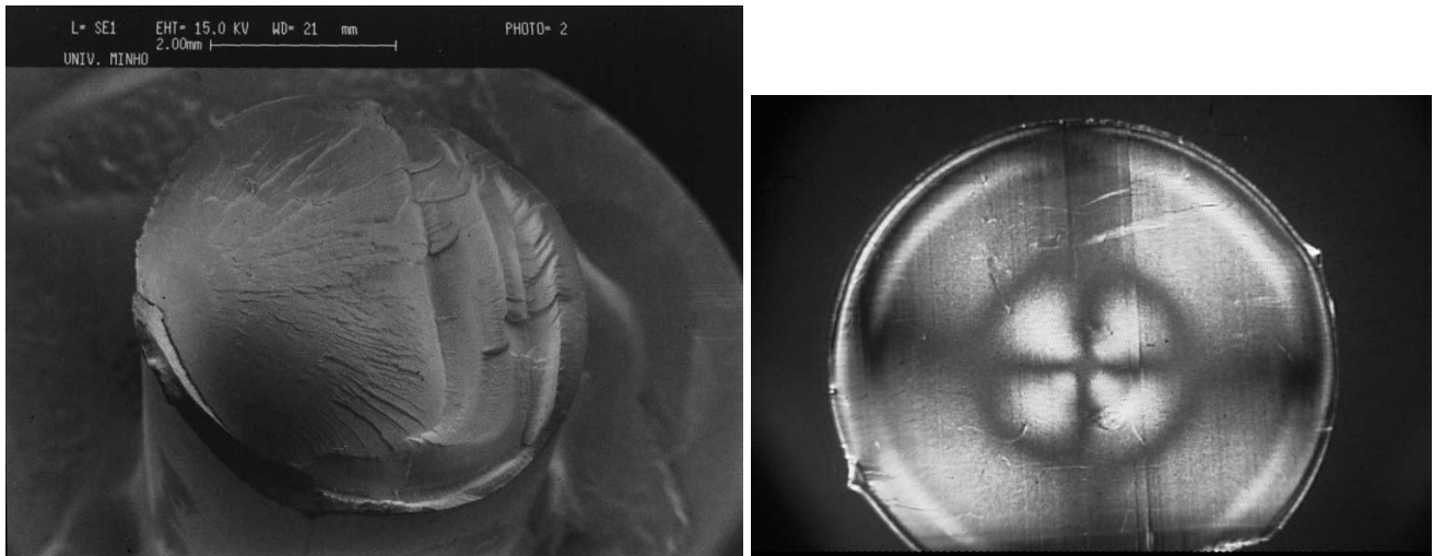
Fig. 2. SEM micrograph of a fracture surface and polarised light microscopy of PEc samples (diameter of the studied samples: 5 mm).
